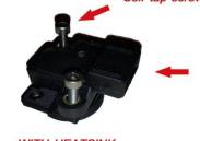
The ignition module can be assembled with or without the heatsink assembly. For a lower profile mount the ignition module amplifier with the metal surface facing downwards and with the connector facing the closed portion of the coil adaptor.
