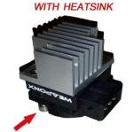
To mount the ignition module with the heatsink mount the ignition amplifier with the labeling upside down, and the metal surface facing up, again with the module connector facing the closed portion of the coil adaptor. Screw in the stainless hardware from the bottom, do not over tighten, snug is all that is required or damage to the plastic adaptor can occur
